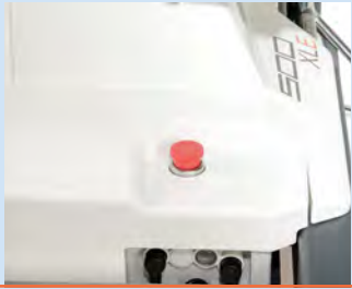
Power supply-independent battery box with integrated emergency stop button.
